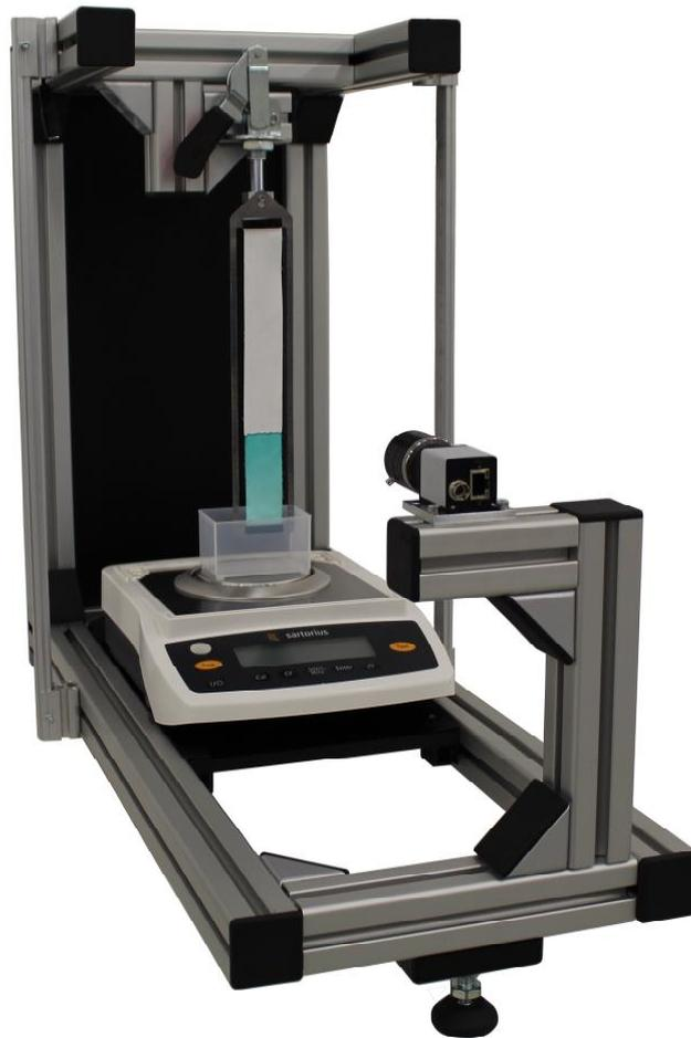
The fluid handling of nonwoven and woven materials for hygienic and other applications involving fluids has a major impact on the functionality of the end product. A detailed analysis of the capillary properties of the material gives essential feedback for purposes of product- and process optimisation.
