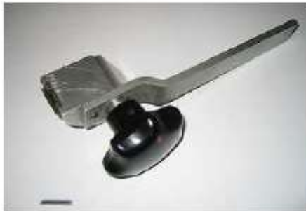
H.2000.28.9 Tool f. opening roller house clip
