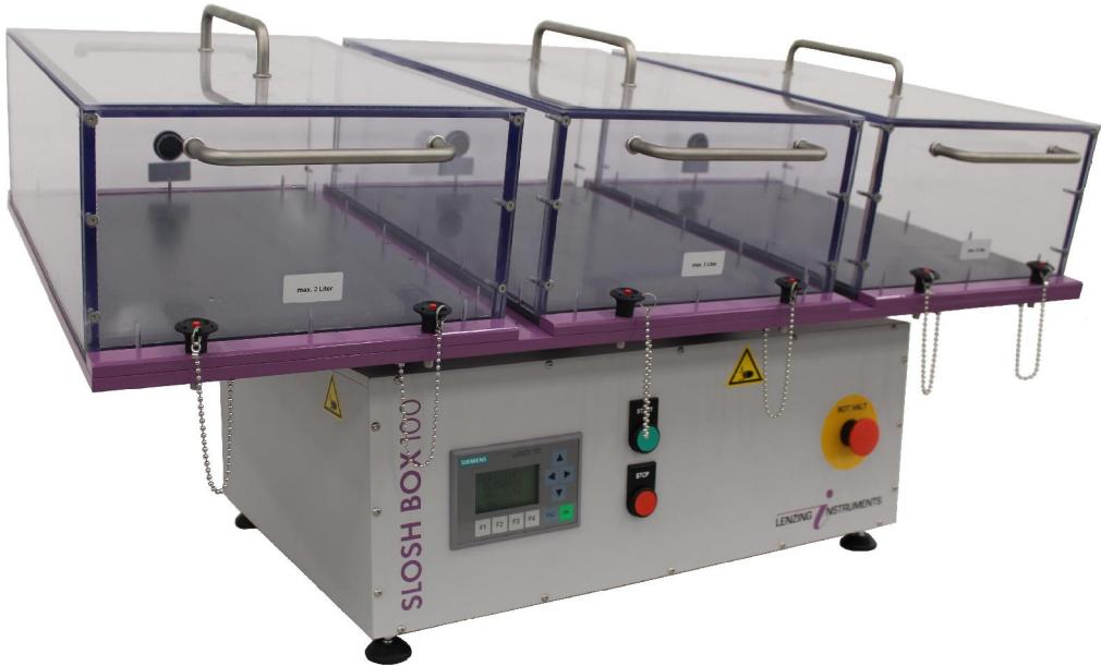
Declaration of flushability becomes more and more important in line with the increasing use of consumable wipes of nonwoven materials. Incorrect or non-existent labelling for flushability causes problems with clogging, blockages and equipment failure in the conveyance and wastewater treatment systems. The guidelines drawn up by INDIA/EDANA include a number of tests, which assist producers in verifying the flushability of their products.
