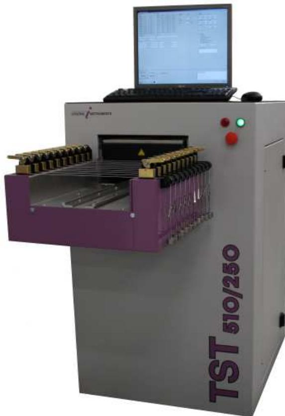
Change of length and shrinkage force at specified temperatures are two dominant quality parameters for technical and industrial as well as for textile filament yarns.
